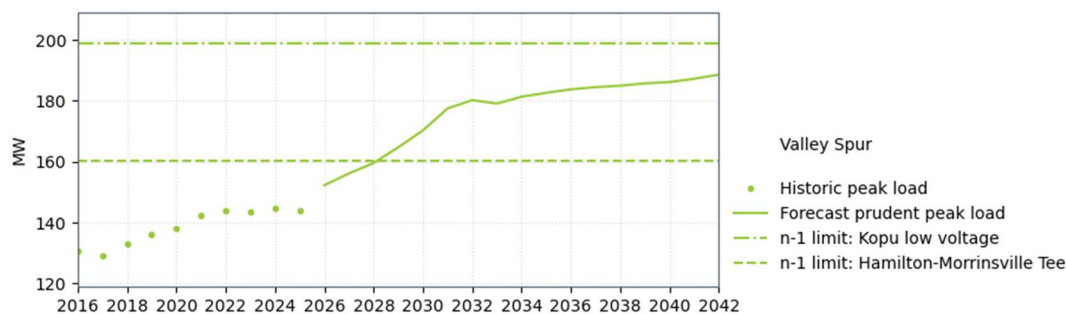
Figure 9-5: Valley Spur circuit capacity
