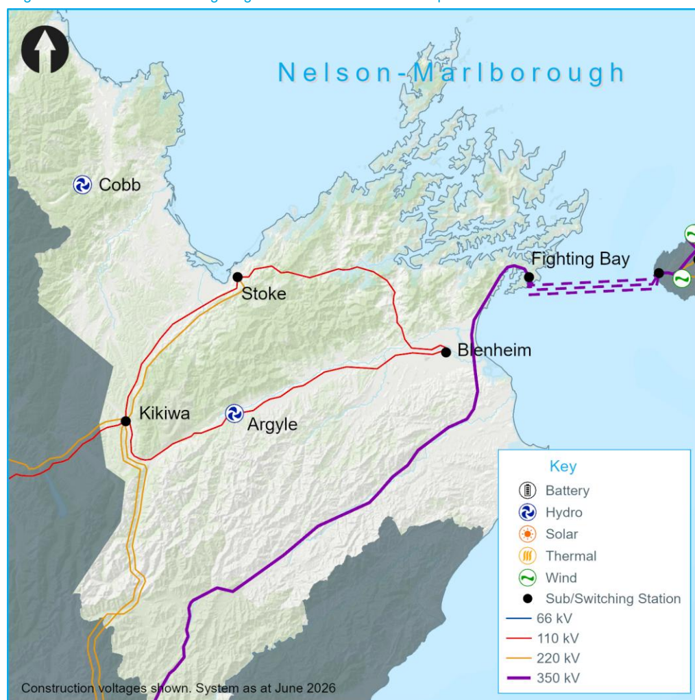
Figure 15-1: Nelson-Marlborough region transmission network map
